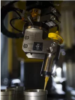
A small robot applies glue to the lens of a missile seeker at Raytheon in Tucson. The lenses can easily be inverted by human engineers, and using the robots helps free up workers from mundane tasks to focus on more complex work that can't be accomplished by machines, officials said. (Photo: Raytheon)
